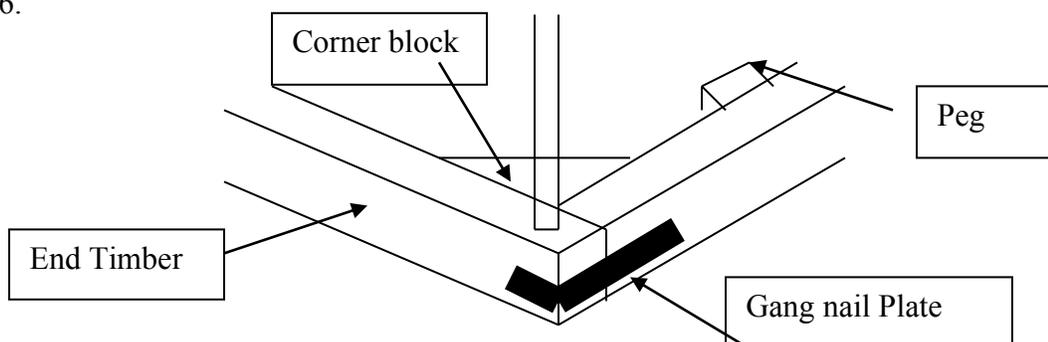
6. Drive pegs on inside of frame until they are flush with the top and nail peg to base timber.
